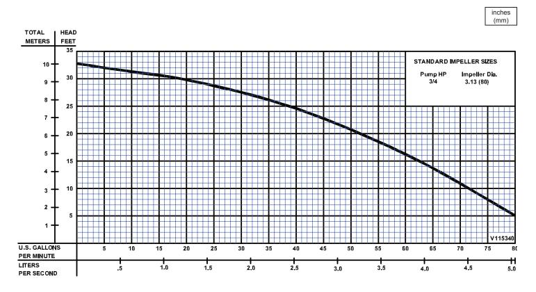
Testing is performed with water, specific gravity 1.0 @  $68^{\circ}$  F @ (20°C), other fluids may vary performance
